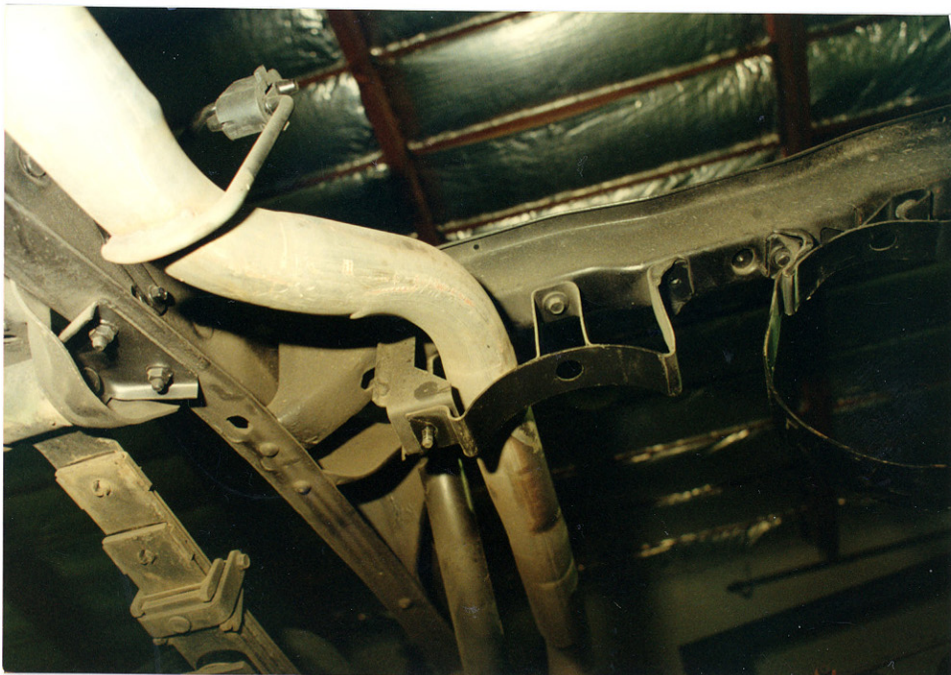
29, 30. Mounting Brackets and Exhaust Pipe Routing Around the Right Side Cylinder
